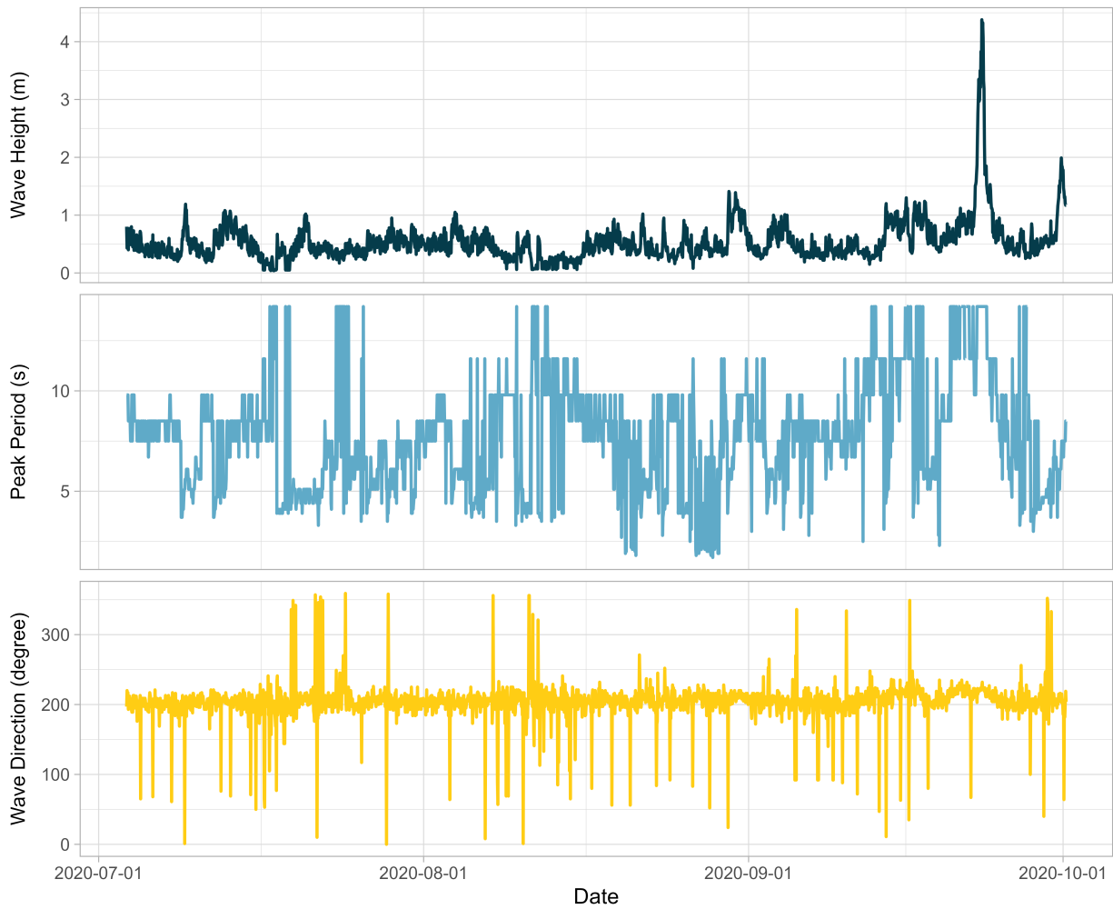
Figure 4: Wave variables over time. Top: significant wave height; Middle: peak period; Bottom: direction wave is travelling from.
