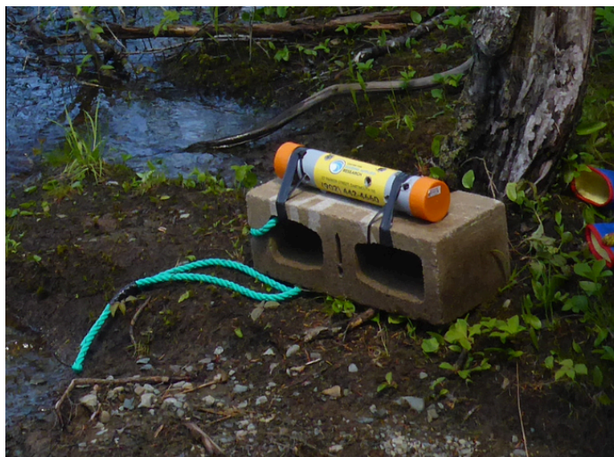
Figure 2: Image of a sensor deployed within a perforated PVC sensor housing attached to a cinderblock anchor.
