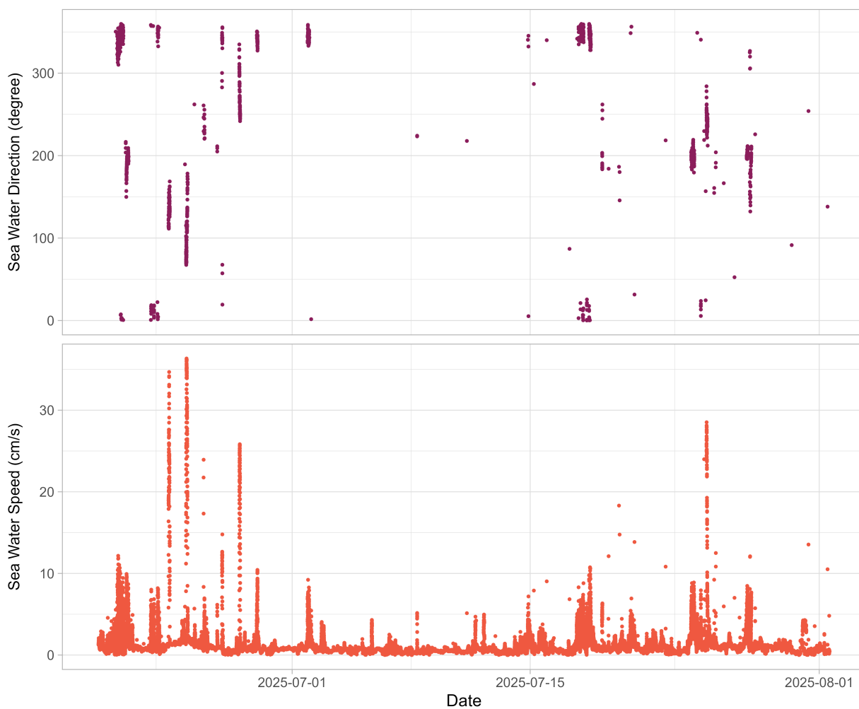
Figure 4: Current variables over time. Top: the direction the current is travelling to; Bottom: current speed.
